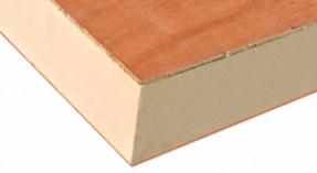
Plylok is a thermal insulation board. Its core consists of rigid polyisocyanurate PIR foam. The board is faced with a gas diffusion tight multilayer foil on both sides and post laminated to plywood on one side.
